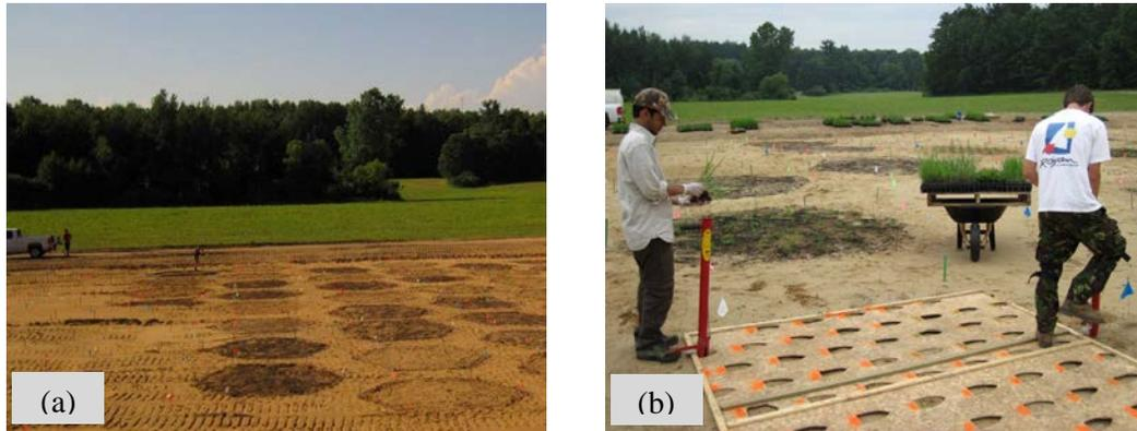
Figure 5: (a) Hexagonal plots with different soil amendments including biochar, compost & biochar and no amendment are ready for planting; (b) Field technicians plant native prairie plugs into the experimental plot.
